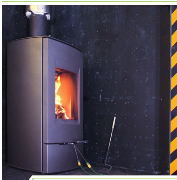
Room heater in the trihedron
