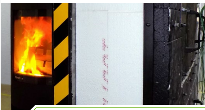
Safety test of a room heater in the trihedron with high thermal insulated walls
