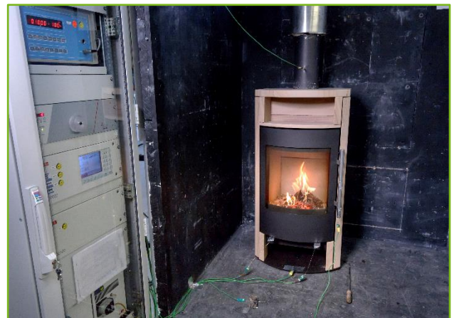
Space heater in the test corner
