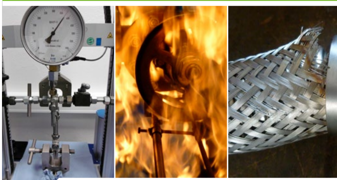
Tensile test pipe connector, Fire-Safe test, burst pressure test (l.t.r.)
